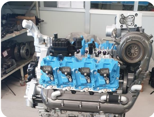
V8 Engine during assembling phase in Italtecnica
