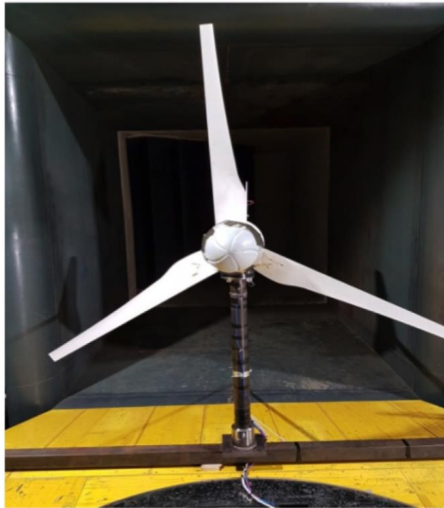
Prototype 1.5 m for wind tunnel testing and field testing
